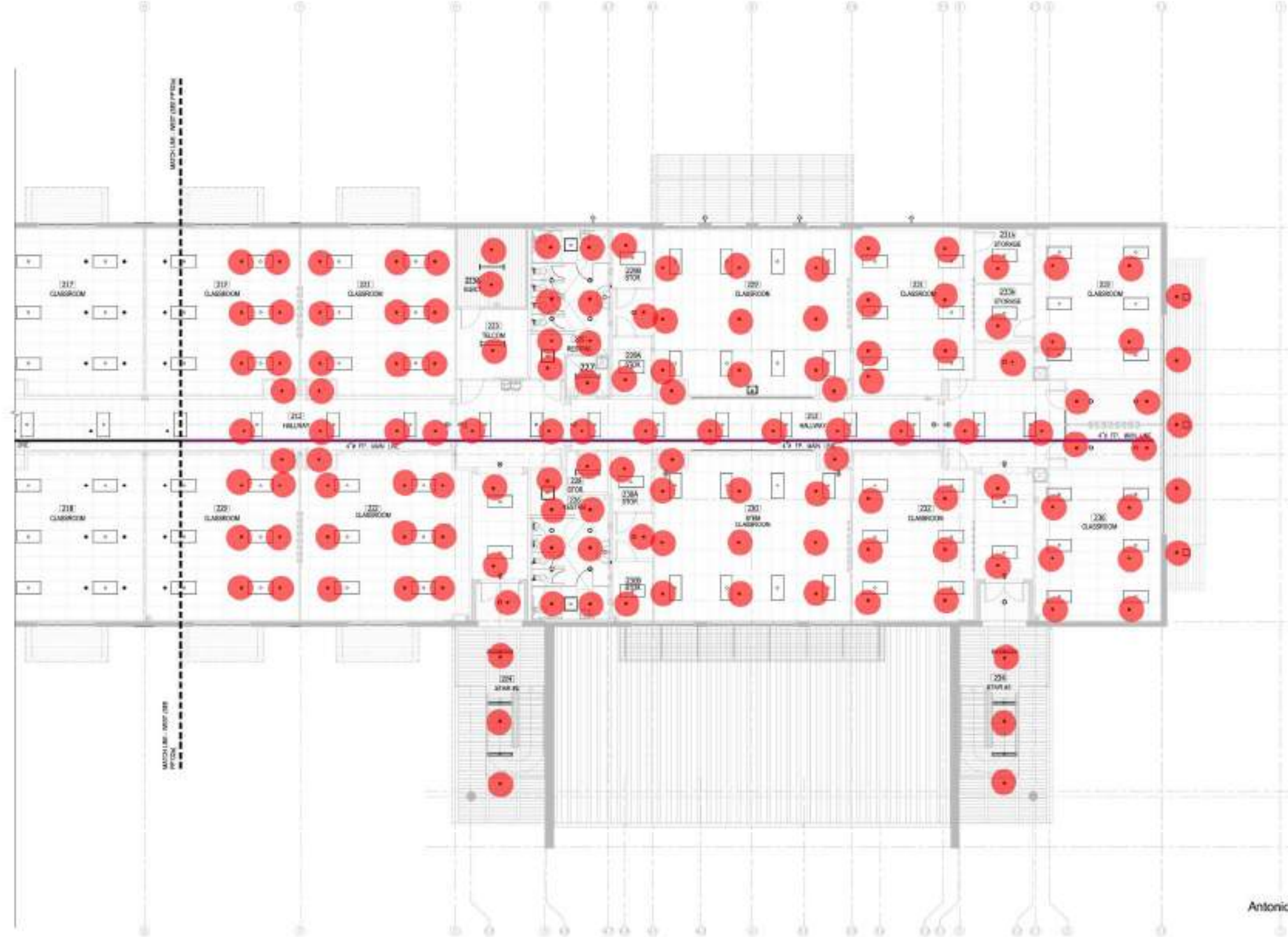
2ND FLOOR FIRE PROTECTION PLAN (EAST)
